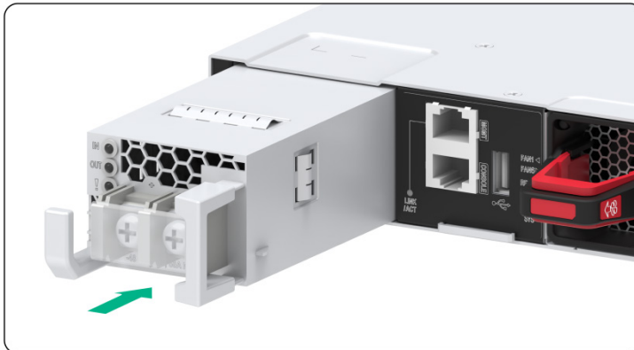
Figure2-54 Installing a PSR2400B-12D-B power supply
