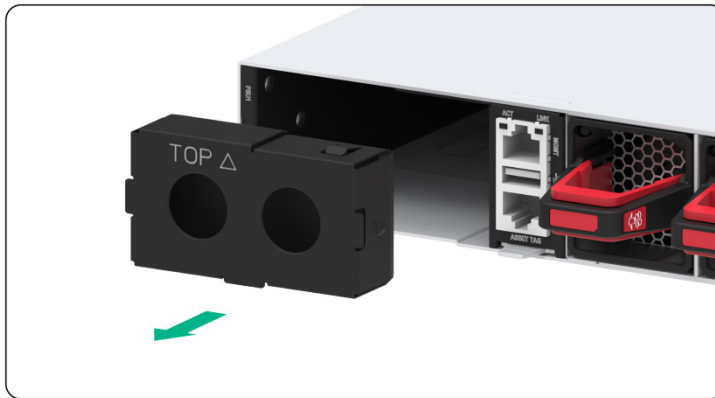
Figure2-51 Removing the filler panel
