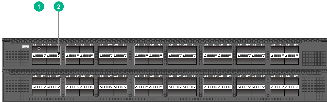
Figure2-1 S9820-64H front panel
