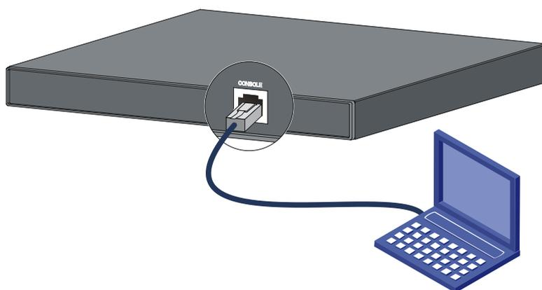
As shown in [Table3-1](#), three types of console cables can be used for connecting the switch to a configuration terminal. The switch is not provided with a serial console cable or a micro USB console cable.
