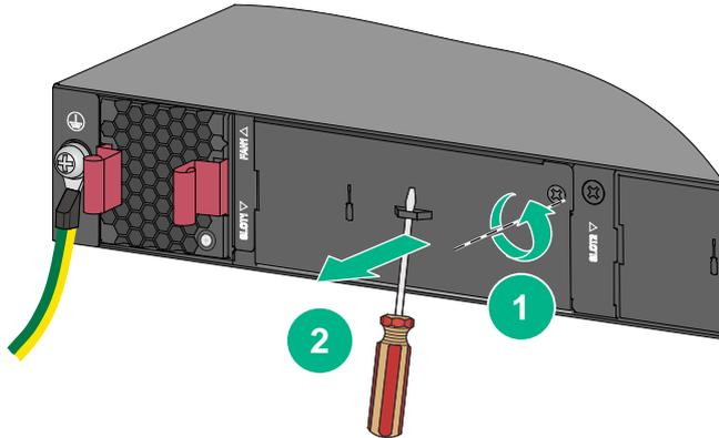
**Figure2-39 Removing the filler panel from the target expansion slot (method 2)**
