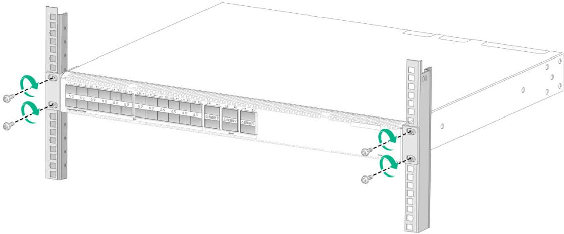
**Figure2-9 Mounting the switch in the rack (power supply-side mounting position for the front mounting brackets, S6520X-30HF-EI switch as an example)**
