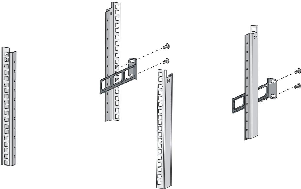
**Figure2-12 Attaching the rear mounting brackets to the rack with the wide flange outside the rack**
