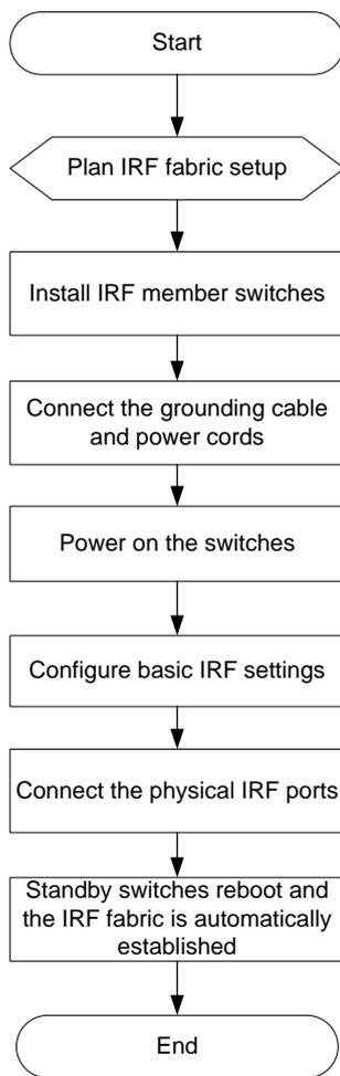
To set up an IRF fabric:
