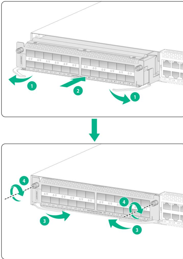
6. (Optional.) If the expansion card does not have an ejector lever, perform the following steps to install it:
