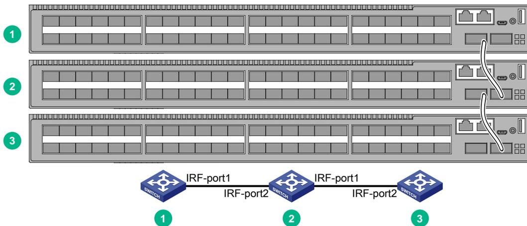
Figure4-3 IRF fabric in ring topology
