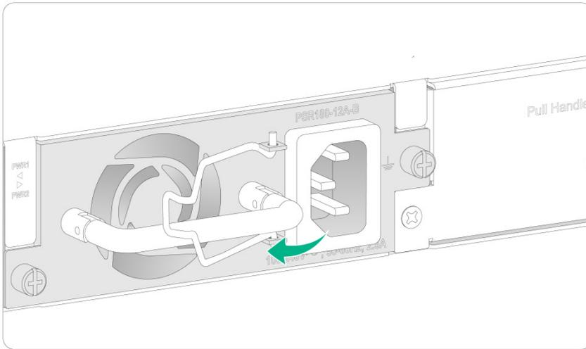
**Figure2-34 Connecting a power cord (2)**
