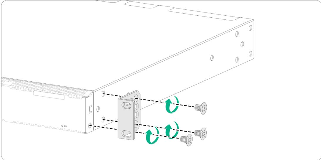
**Figure2-7 Attaching the front mounting brackets to the power supply-side mounting position (S6520X-30HF-EI switch as an example)**
