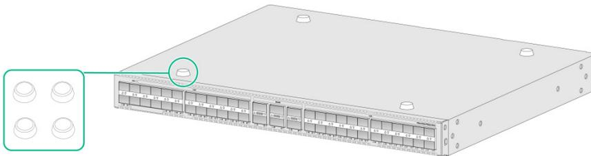
Figure2-16 Mounting the switch on a workbench (2) (S6520X-54HF-EI switch as an example)
