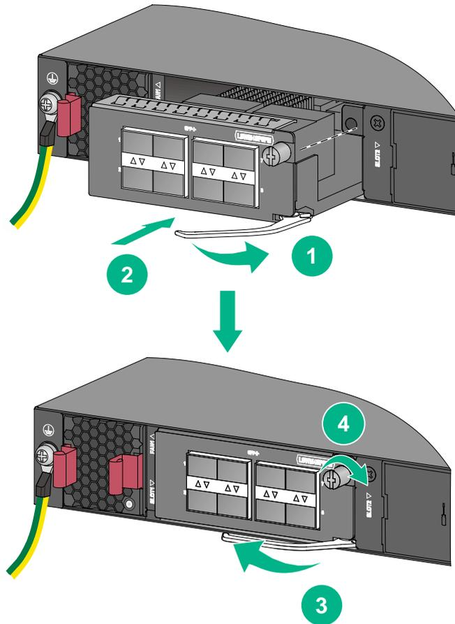
5. (Optional.) If the expansion card has two ejector levers, perform the following steps to install it:
