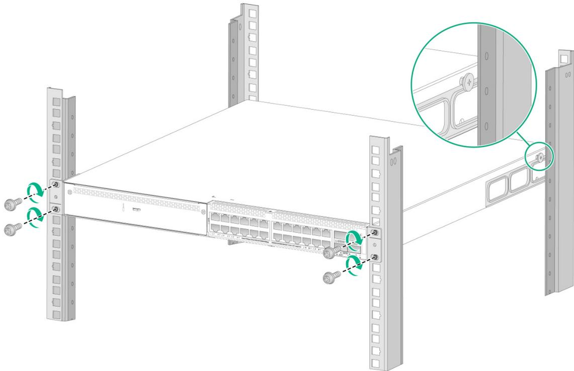
**Figure2-14 Mounting the switch in the rack (with the wide flange of the rear mounting brackets outside the rack)**
