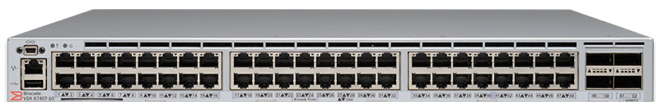
Figure 3: The Brocade VDX 6740T-1G Switch provides 48 1000BASE-T/10GBASE-T ports and four 40 GbE QSFP+ ports.
