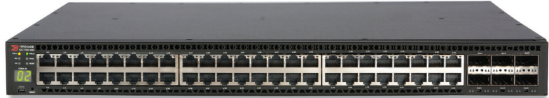
Figure 2: The Brocade ICX 7750-48C features 48 10GBASE-T ports and 6 40 GbE QSFP+ ports that can be split into 24* 10 GbE SFP+ ports.
