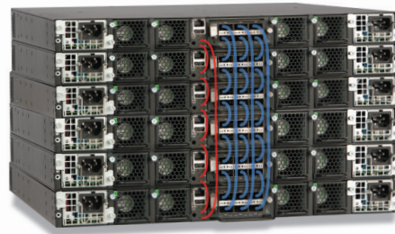
Figure 4: Up to 12 Brocade ICX 7750 Switches can be stacked using up to six standard full-duplex 40 Gbps QSFP+ ports per switch, providing up to 2,880 Gbps of aggregated stacking bandwidth. Two 1 Gbps ports on each switch can be used to create a dedicated path for forwarding system health and control information across the stack for maximum reliability.
