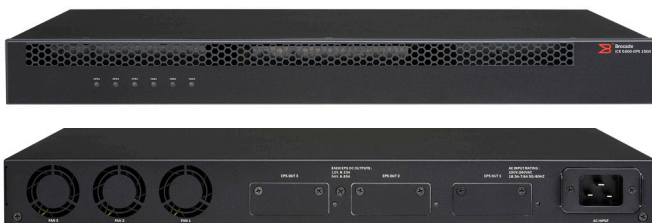
Figure 3: The optional Brocade ICX 6400-EPS150 is an external power supply source to provide additional power to the Brocade ICX switches (except the Brocade ICX 6430-C, 6450-C, and 6430-24). It also can be used for system power redundancy and increased PoE/PoE+ power budget to enable additional PoE/PoE+ ports. Each Brocade ICX 6400-EPS150 can connect up to three Brocade ICX 6430 and 6450 Switches.
