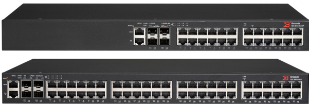
Figure 1: Brocade ICX 6450 Switches support four dual-mode 1 GbE/10 GbE SFP/SFP+ ports for uplink and stacking, and up to 48 1 GbE RJ-45 ports. Brocade ICX 6430-24 and 6430-48 Switches support four 1 GbE SFP ports for uplink and stacking to provide a cost-optimized solution for lower-traffic networks.
